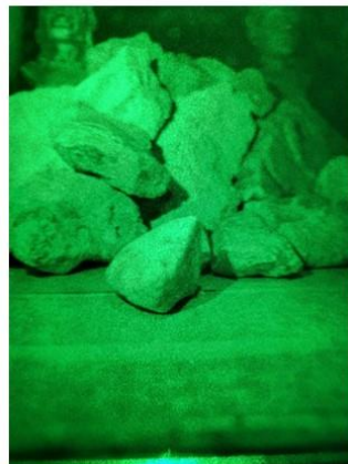
Figure 11. This is the resulting hologram from the setup shown in figure 10. It is reconstructed with a green laser diode.
