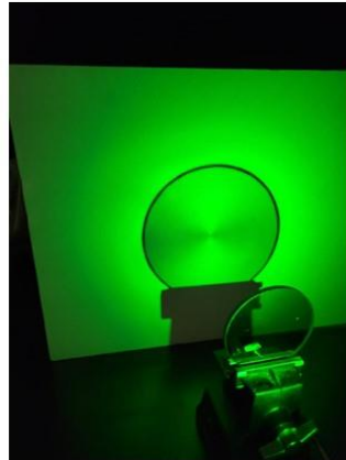
Figure 8. Short 3mm fibers maintain some polarization as indicated by the two faint dark triangular projections after passing through the axis finder in the foreground. The polarization axis can be rotated by twisting the fiber.
