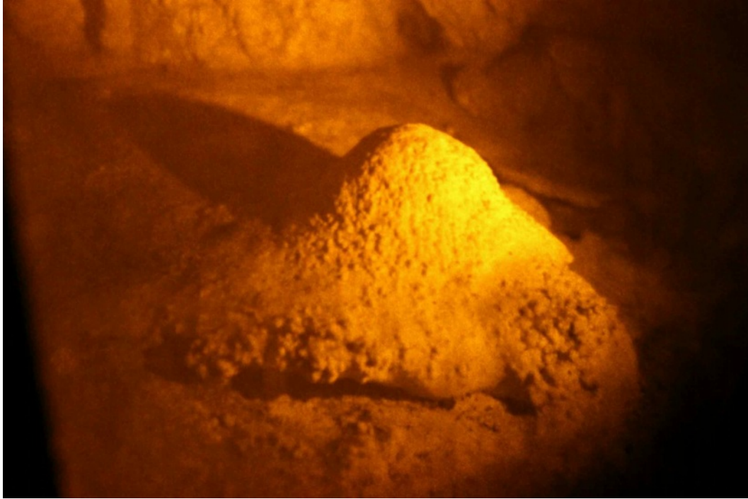
Figure 4. A typical cave transmission hologram made with a C315M laser reconstructed with a 594 nm HeNe laser.
