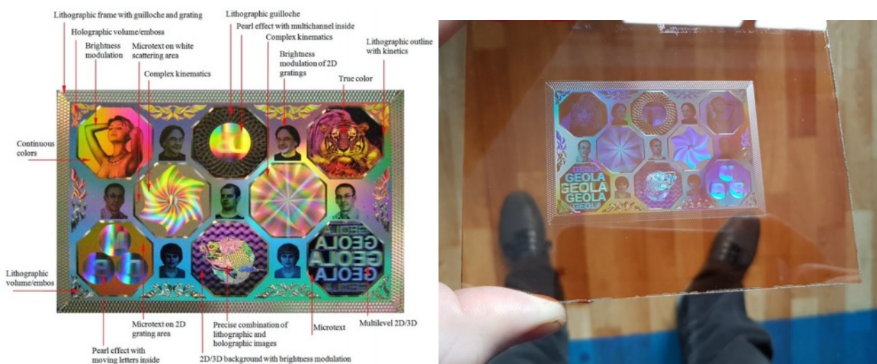
Figure 8: Described diffractive features (Left) and the actual photoresist master producible by IMP-6 (Right)
