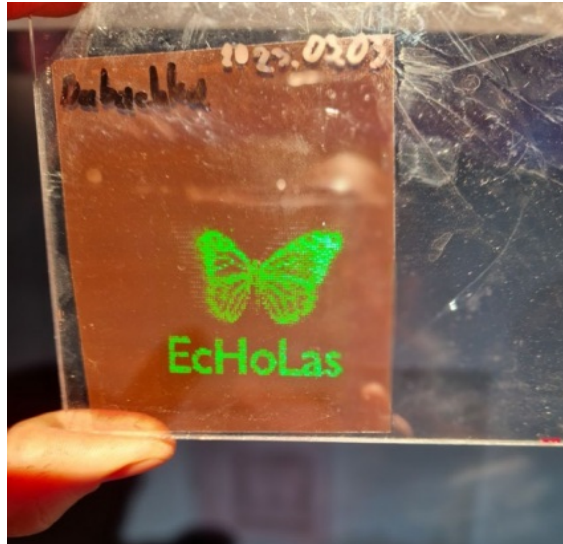
Figure 17: A first small DWDH full parallax hologram created by the printer shown in figure 16 on HX200 photopolymer.
