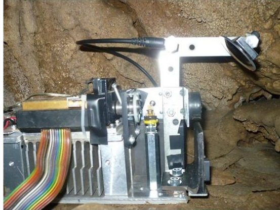
Figure 2. This is an example of a C315M device using a 1mm fiber and a convex mirror in place of a spatial filter.
