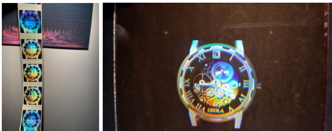
Figure 5: Full-Parallax Optically-Variable Hologram Labels (Left) and Master (Right). Digital DWDH Master made using DIWO-6 originator on photoresist.
