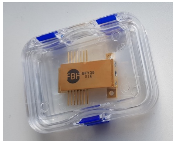
Figure 3: An example of a 632 nm Echolas laser produced by Echolas partner FBH
