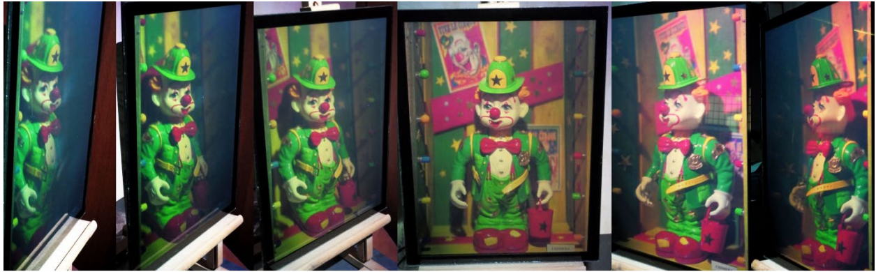
Figure 2. 30×40 cm CHIMERA™ 180° hologram illuminated with an RGB LED. The hologram presents a complete 180 degree horizontal field angle.
