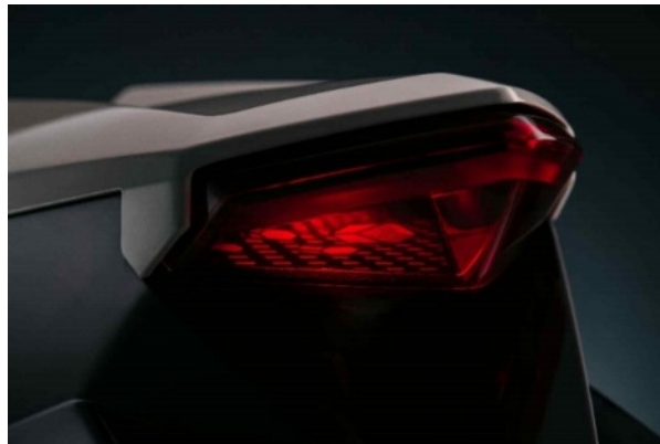
Figure 6. Photograph of the prototype motorbike backlight. Realized with a lightguide with zero order dumping.
