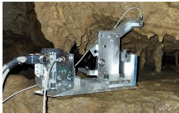
Figure 6. This PL530 device uses a 1 mm fiber to direct the reference beam and eliminate the spatial filter. The variable beamsplitter was replaced with a fixed ratio beamsplitter to further simplify it.
