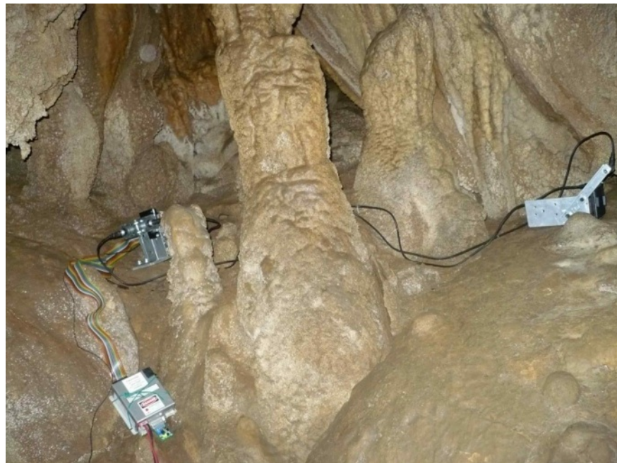
Figure 3. A setup with the holography head separated from the laser with fibers carrying the reference and object light.
