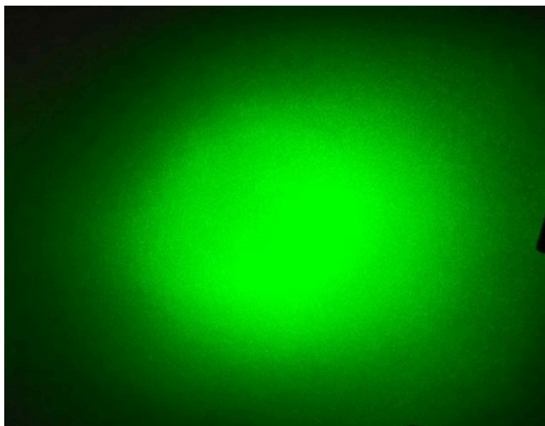
Figure 7. The output of a 3mm fiber has a few artifacts but is clean enough to be used for a reference beam.
