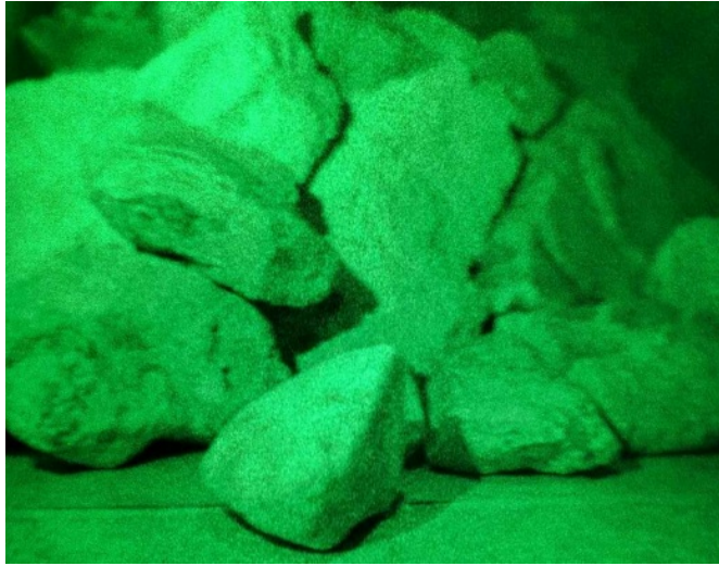
Figure 11. This is the resulting hologram from the setup shown in figure 10. It is reconstructed with a green laser diode.
