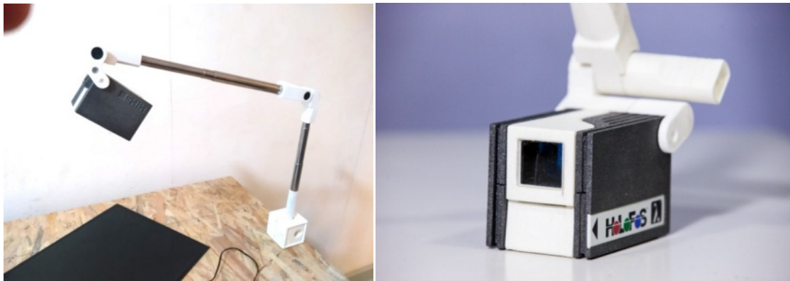
Figure 6. The HoloFoS- \lambda mounted on a tabletop and a close up of the LED head of the device.
