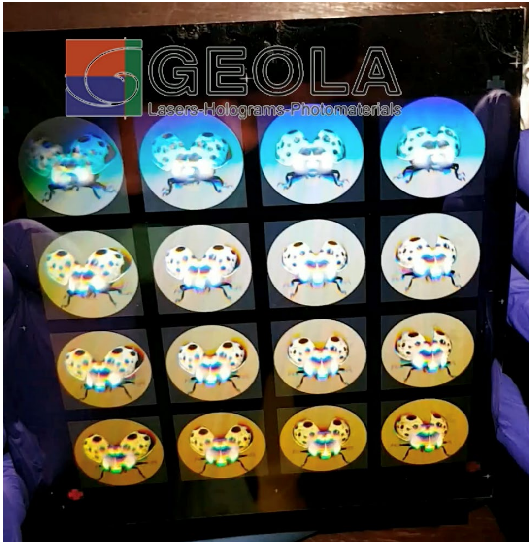
Figure 13: The full parallax "LadyBug" data of Figure 9 produced on DIWO-6 originator using optical recombination. Later said holographic master plate was transferred to nickel via traditional electroforming.
