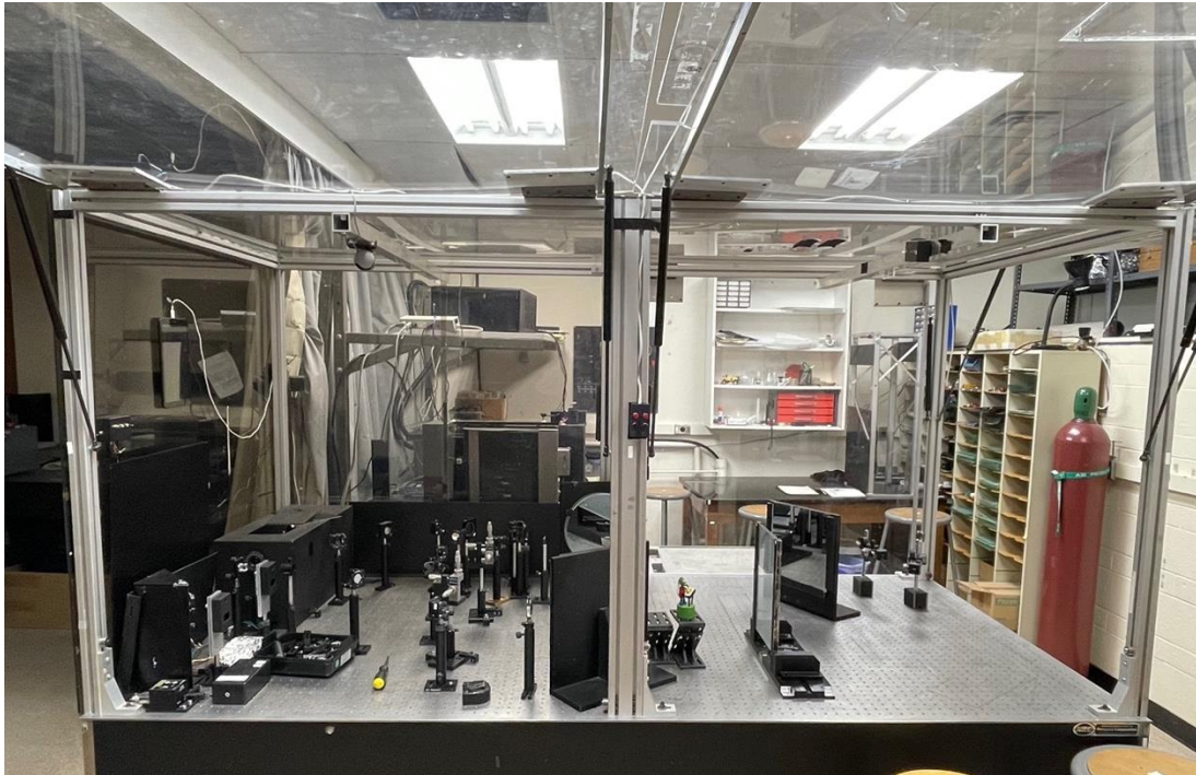
Figure 1. The optical table with an enclosure above to limit air currents. In this photograph, the enclosure doors are open, and they can be seen at the very top of the image (they are lifted up).
